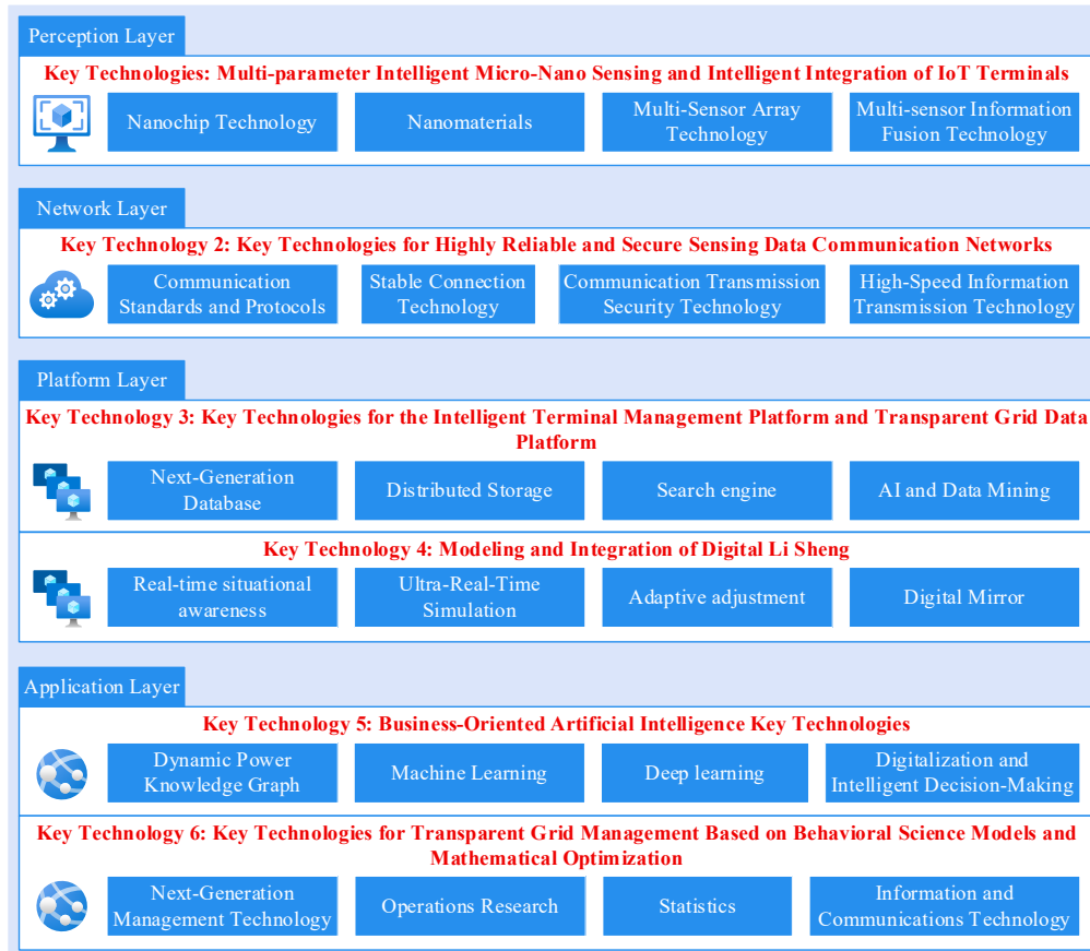
Figure 1. The overall framework of the transparent grid technology system.
