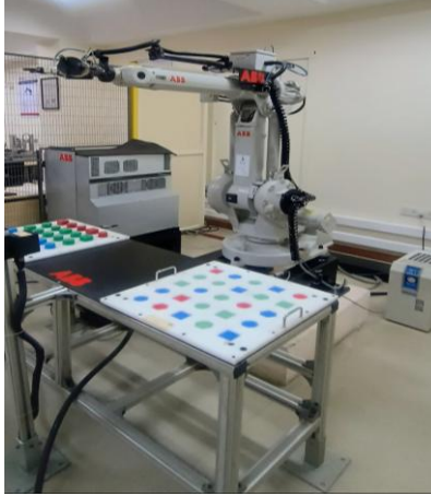
Fig. 3. ABB IRB 1410 manipulator with the dual-pallet workstation. The IRC5 controller (left) communicates with the host PC over Ethernet/IP for real-time trajectory commands.
