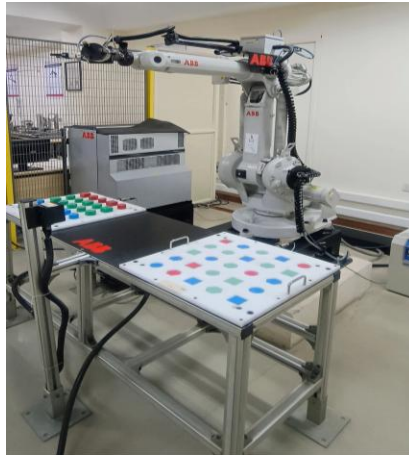
Fig. 4. Alternate view of the workstation showing the spatial relationship between the manipulator, the controller cabinet, and the dual pallets. The vision camera (not visible here) is mounted on a pole at the right corner.
