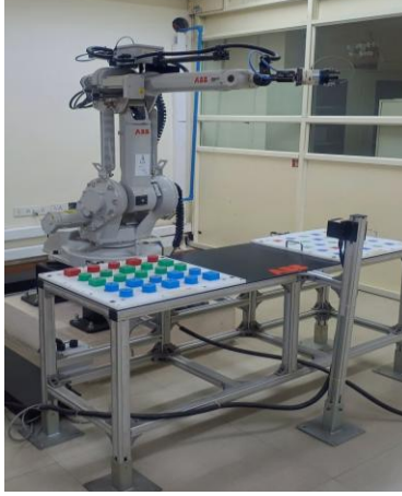
Fig. 5. The manipulator end-effector approaches Pallet A (in front, 3-D coloured pegs), with Pallet B containing multi-shape flat targets in the background. The vision pole is on the right.
