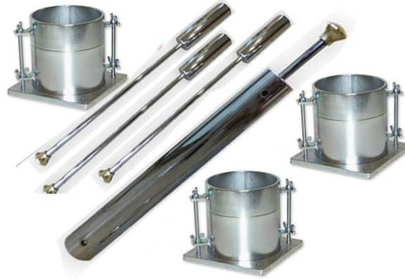
Figure 1. Modified Proctor test setup
