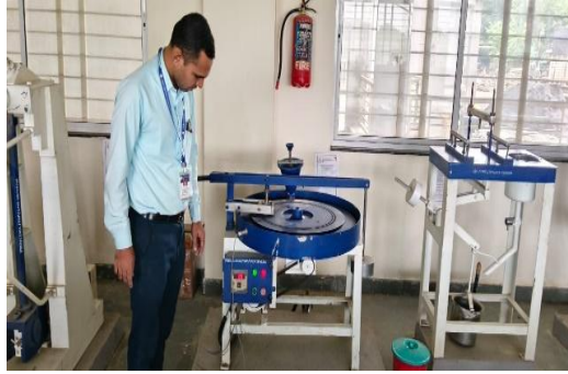
Figure 13. Abrasion test on ROCC
