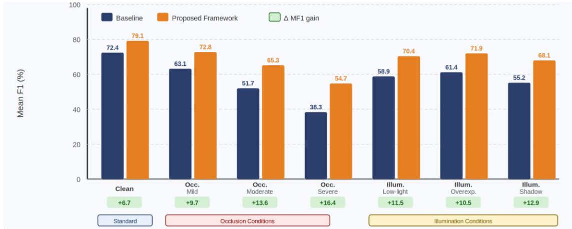
Figure 3: Mean F1 comparison across all challenging evaluation conditions. Green annotations show absolute MF1 gain of the proposed framework over the baseline. Gains increase with occlusion severity, peaking at +16.4 for severe occlusion.
