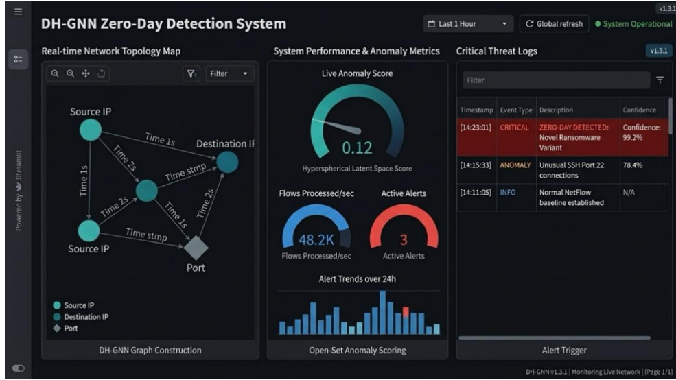
Figure 4. Real-time inference dashboard demonstrating the live visualization of dynamic graph topologies, continuous anomaly scoring, and automated zero-day alert generation for security analysts.
