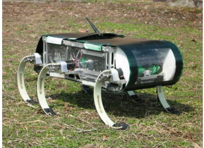
**Figure. 3:** RHex. A six-legged robot with only one degree of freedom. The robot moves exceeding five body lengths per second (2.7 m/s), climbs slopes exceeding 45 degrees, swims, and climbs stairs.
