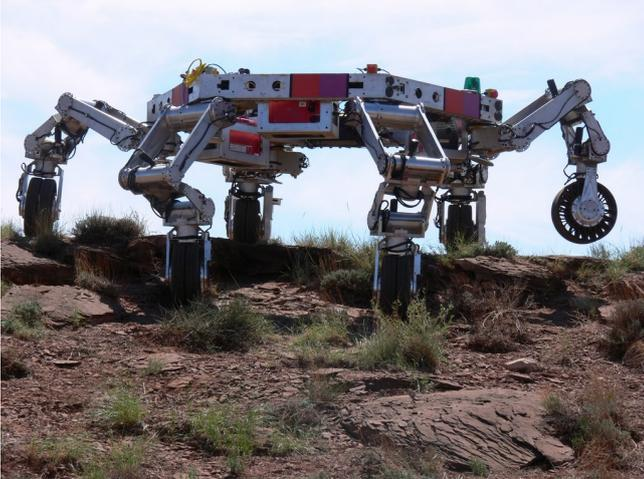
**Figure. 1:** ATHLETE. This six-legged robot was designed by NASA for exploration of planets, especially of Mars [4].
