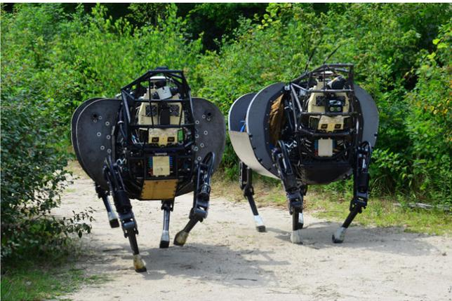
**Figure. 2:** LS3. A four-legged robot developed by Boston Dynamics for military purposes. The robot can reach the speed of 10 km/h.
