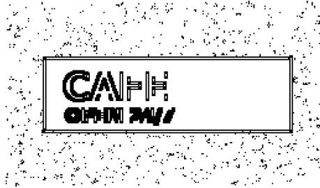
Figure. 6 Stage 5 output: fused Sobel edge map after thresholding; text strokes retained, smooth background suppressed
