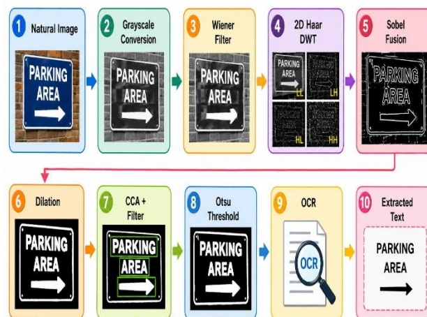
Figure. 1 Block diagram of the proposed 2D Haar DWT scene text extraction pipeline
