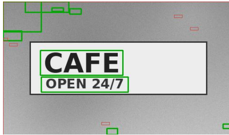
Figure. 8 Stage 7 output: connected components after geometric filtering (green = accepted text, red = rejected non-text)
