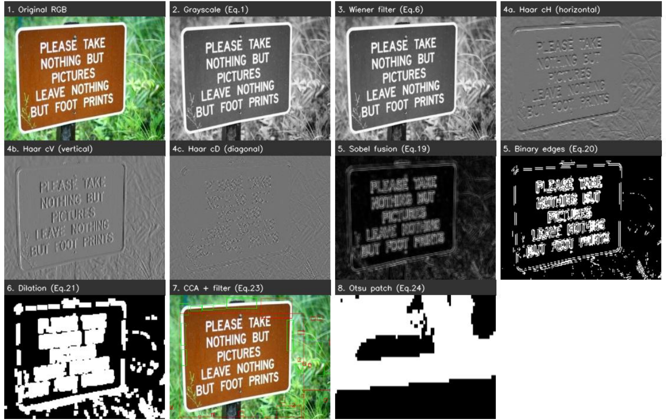
Fig. 2. Stage-by-stage pipeline output for the park sign (text.png): original, grayscale (Eq. 1), Wiener filtering (Eq. 6), Haar detail sub-bands cH, cV and cD (Eqs. 11–13), Sobel sub-band fusion (Eq. 19), binary edge map (Eq. 20), morphological dilation (Eq. 21), connected-component filtering with the geometric density ratio (Eq. 23; green = accepted text, red = rejected), and an Otsu-binarized patch (Eq. 24).
