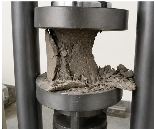
Fig. 7. Cube specimen at failure under compression.
