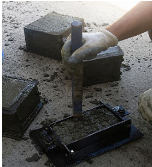
Fig. 3. Compaction of concrete specimens.
