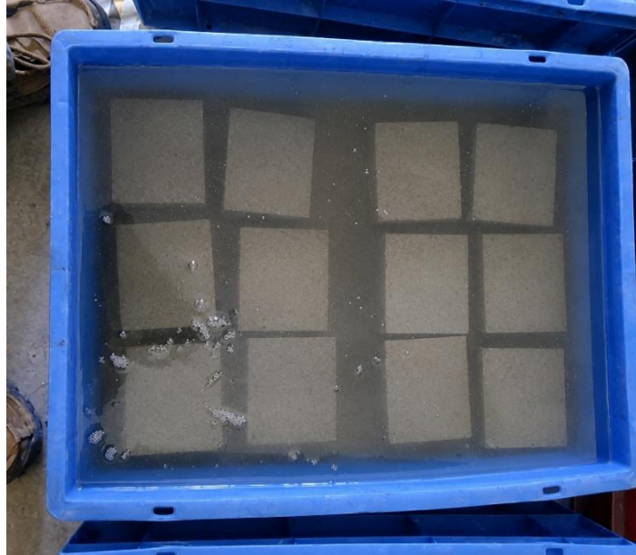
Fig. 4. Water curing of cube specimens.
