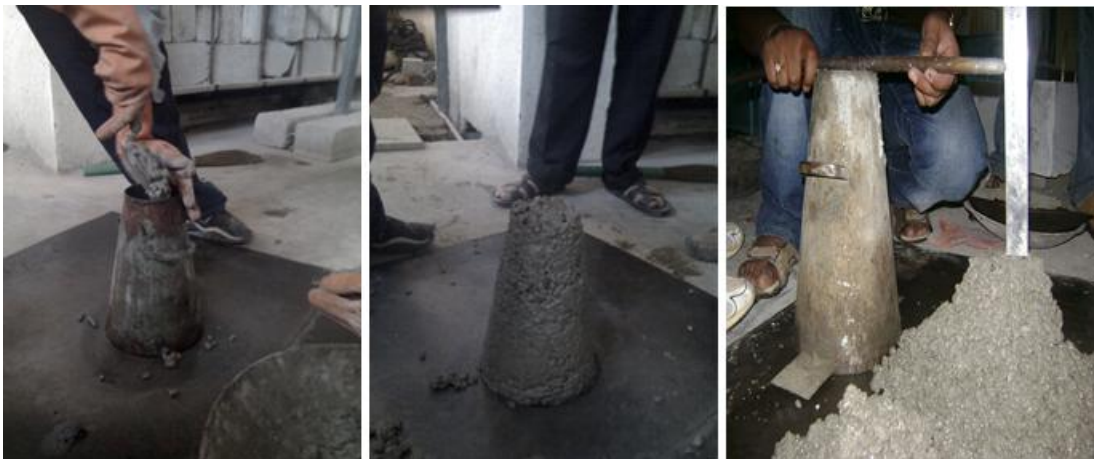
Fig. 5. Slump-cone test on fresh concrete.
