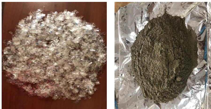
Fig. 1. (a) Waste-plastic strips cut from recycled PET bottles; (b) Class-F fly ash used as the pore-filling admixture.
