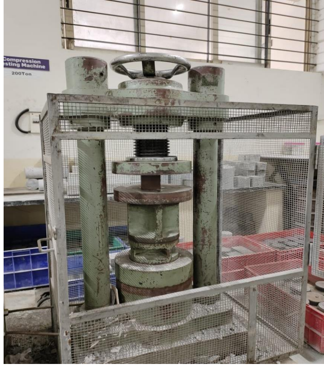
Figure 6. Compression testing machine set-up used for cube compressive-strength determination. 10
