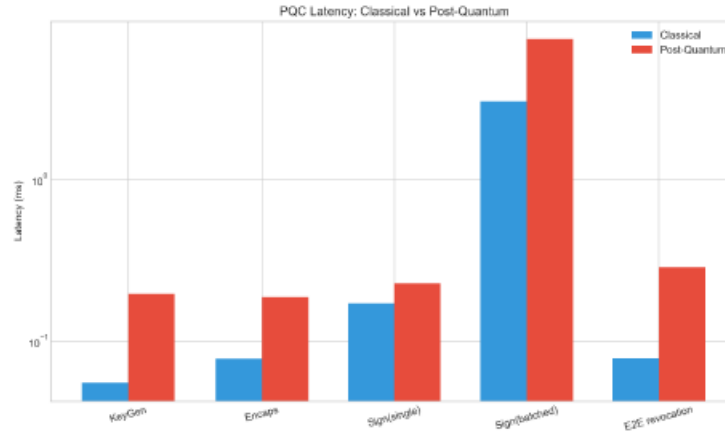
Fig. 4. Classical vs. post-quantum operation latency comparison
