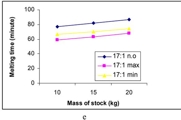
Figure 7. Effect of mass on melting time at each a/f ratio
