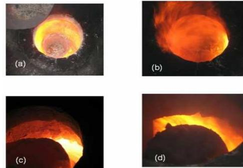
Figure 12. Types of Non-oscillating combustion flames.
