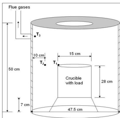
Figure 4. Schematic Temperature distribution in the furnace
