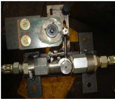
Figure 3. Oscillating combustion valve
