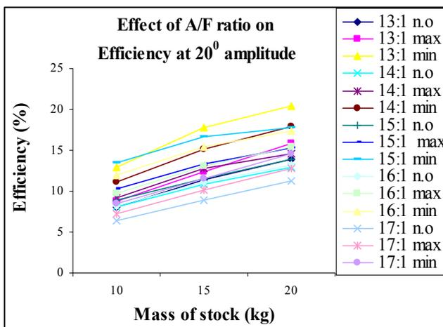
Figure 10. Effect of a/f ratio on efficiency
