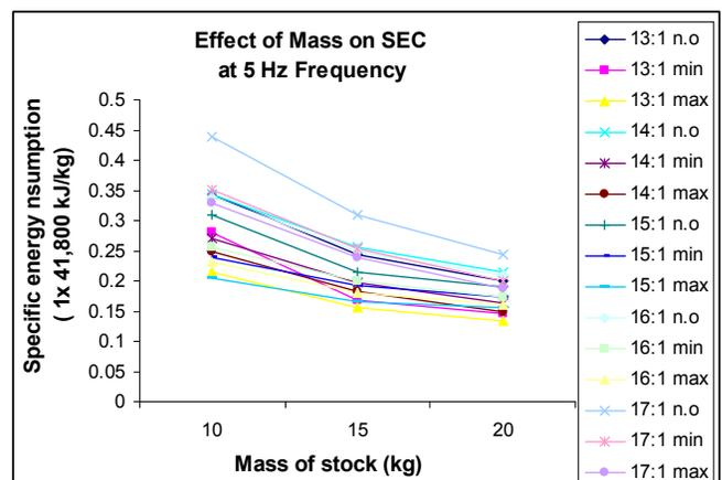
Figure 8. Effect of mass on specific energy consumption
