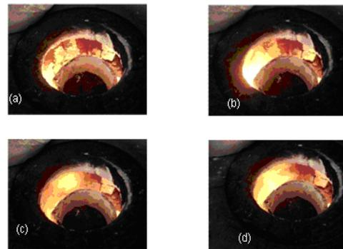
Figure 13. Types of oscillating combustion flames.
