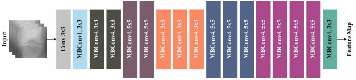
Fig. 2. Framework of EfficientNetB0 with MBConv4
