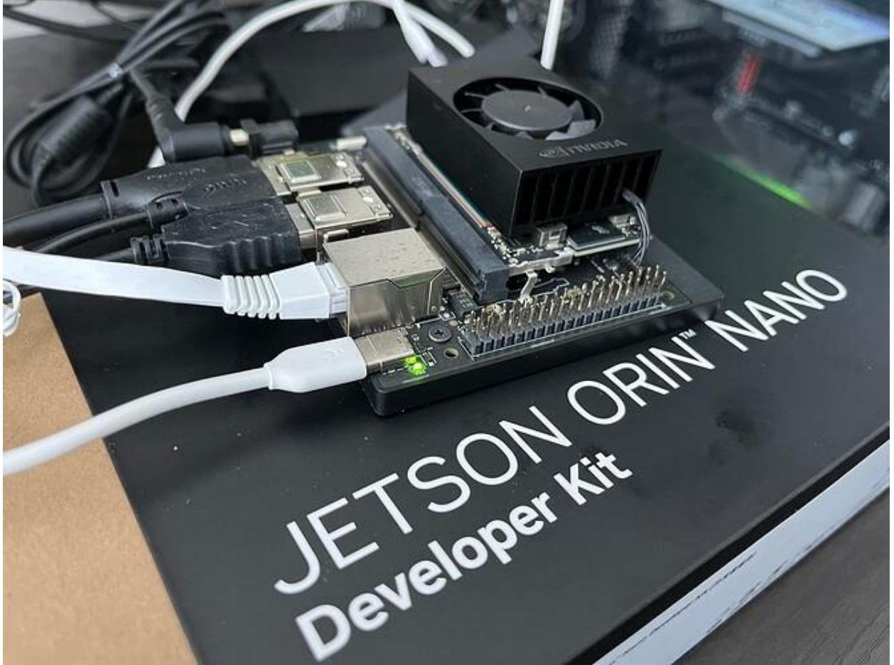
Figure 2: NVIDIA Jetson Orin Nano Developer Kit used for all benchmarking experiments. The sub-USD-200 embedded platform provides a complete TensorRT software stack (CUDA 11.4, cuDNN 8.6, TensorRT 8.5) within a 15 W MAXN power envelope.
