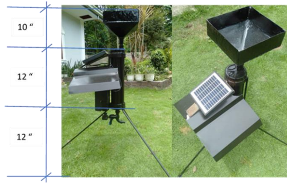
Figure 3. Height Dimension of the Automated Rainfall Measurement Device
