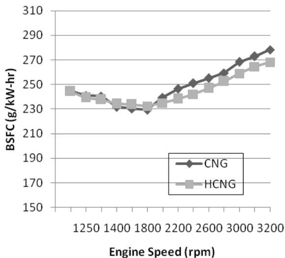
Figure 4. BSFC Comparison of CNG and HCNG engine
