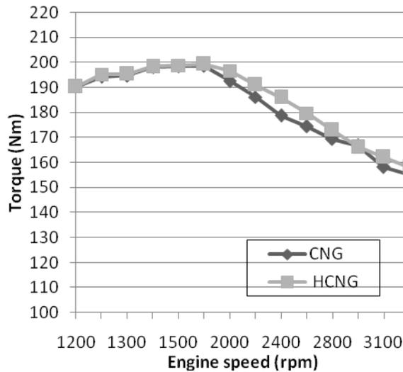
Figure 3. Torque comparison of CNG and HCNG engine
