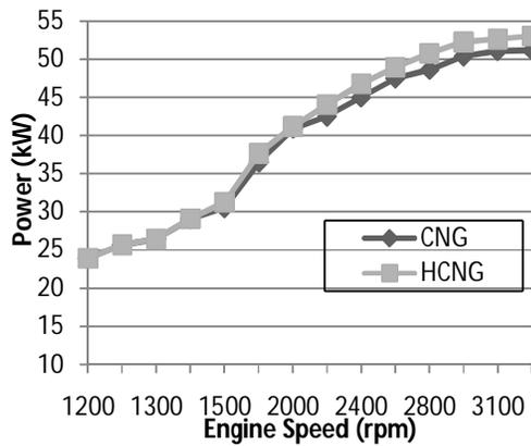
Figure 2. Power Comparison of CNG and HCNG Engine
