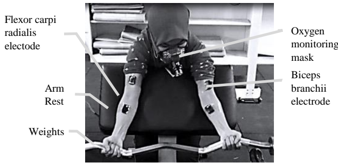
Figure 1. The sEMG signal data collection setup for isotonic muscle contractions.
