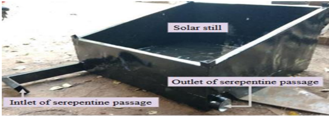
Fig. 6 Outlet and Inlet of Serpentine Passage Beneath the Basin of Solar Still
