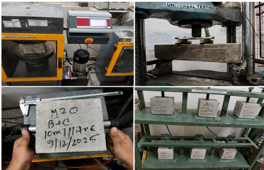
Figure 6: Compressive Strength Test, Flexural Strength Test, Ultrasonic Pulse Velocity Test, Water Penetration Test
