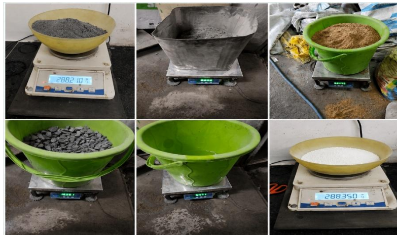
Figure 3: Rice Husk Ash, 43 grade Ordinary Portland Cement (OPC), Fine Aggregates (Zone II), Coarse Aggregate (10 mm and 20 mm size), Potable Water, Calcium Lactate (2%) as Nutrient
