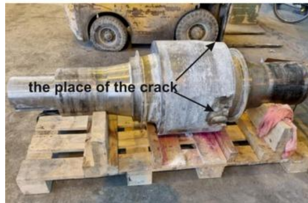
Figure1.1: (a) Shaft of the two-roller mill with a damaged ring, showing one of the two damage locations; (b) Shaft of the two-roller mill with a damaged ring, rotated to reveal the second damage location.
