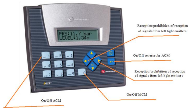
Fig. 11. Purpose of PLC control buttons. ACM = Automatic Control Mode; MCM = Manual Control Mode.
