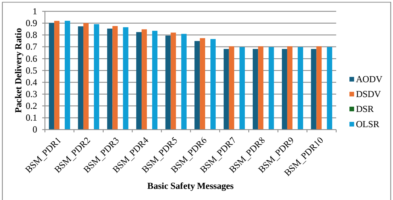
Figure 10: Basic Safety Messages Packet Delivery Ratio Analysis
