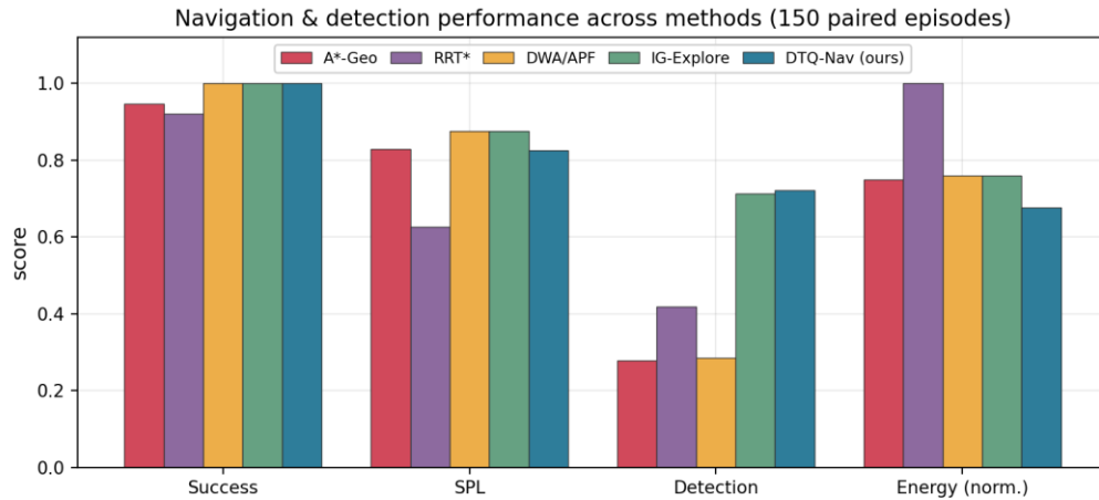
Figure 5. Navigation and detection performance across methods (150 paired episodes). DTQ-Nav matches the best success and detection rates while achieving the lowest normalized energy. Energy is normalized by the maximum across methods.
