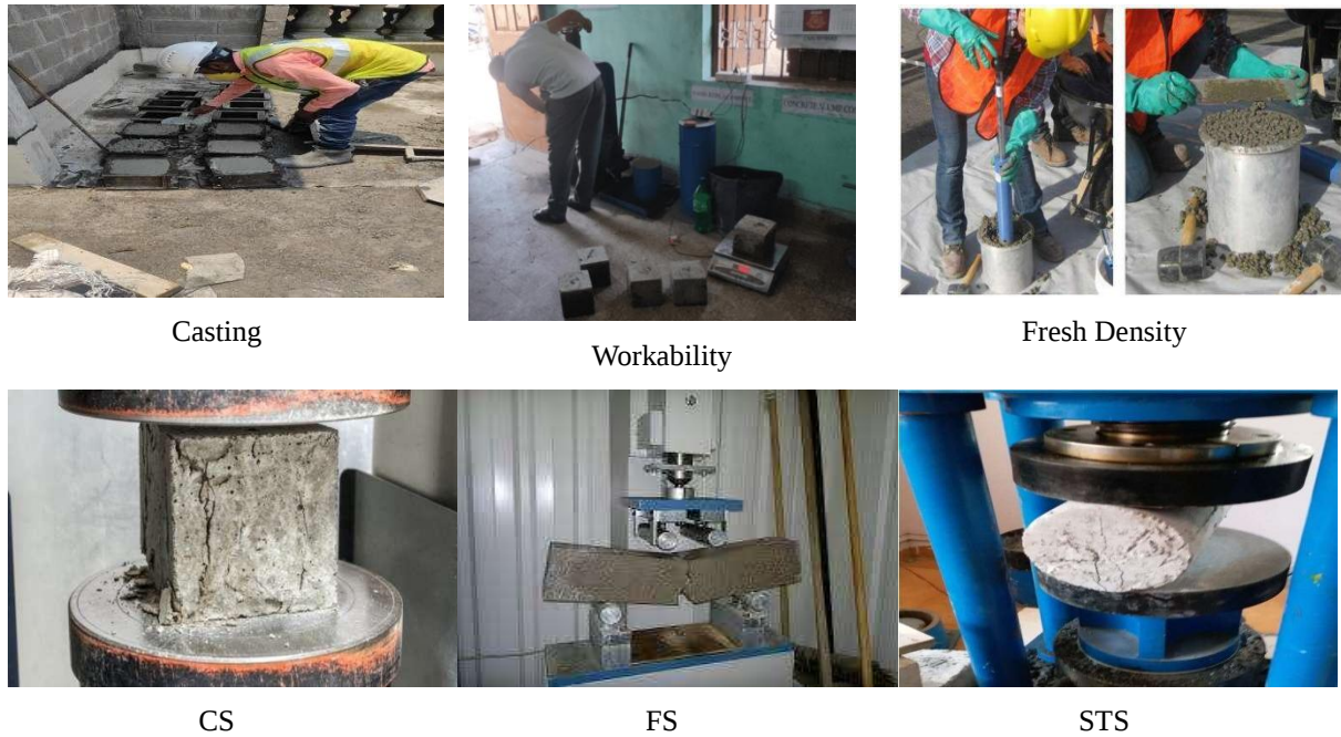
Figure 8: Casting and testing of concrete
