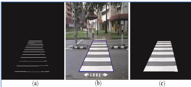
Figure 8 Examples of pedestrian crossing region detection: a) candidate increasing HE segment of a pedestrian crossing, b) detected ROI in the original PC image, and c) detected pedestrian crossing region.
