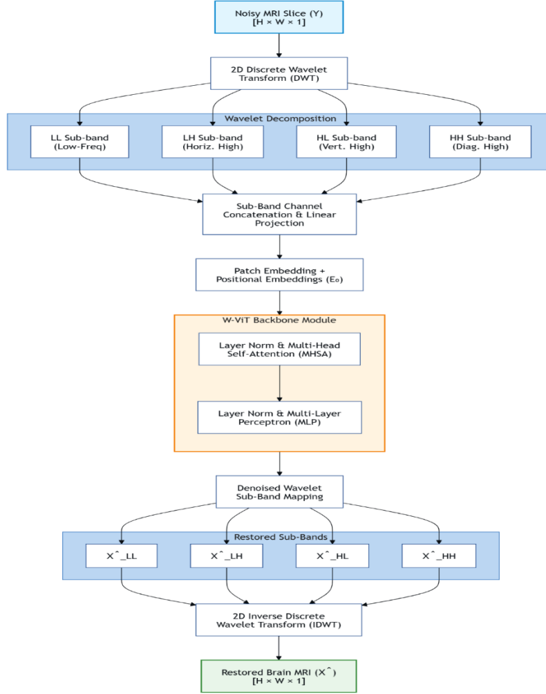
Fig. 1: General schematic architecture of the proposed Wavelet-Informed Vision Transformer (W-ViT) framework. The noisy input MRI slice Y is decomposed by 2D DWT into four sub-bands (LL, LH, HL, HH) and processed by Transformer Encoders with Multi-Head Self-Attention and reconstructed by Inverse DWT (IDWT) to obtain the restored MRI \hat{x} .
