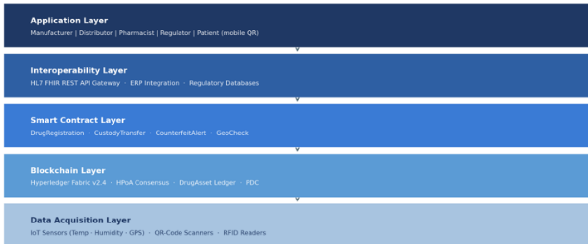
Figure 1. PharmChain Five-Layer Architecture
