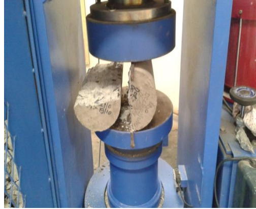
Fig. 21 Sample test on Split tensile test apparatus
