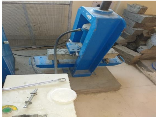
Fig. 19 Sample test on Flexural Strength test apparatus
