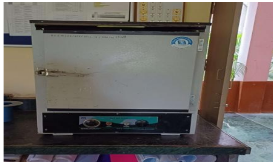
Fig. 9 Oven for oven curing
