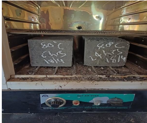
Fig. 10 Samples kept for Oven Curing
