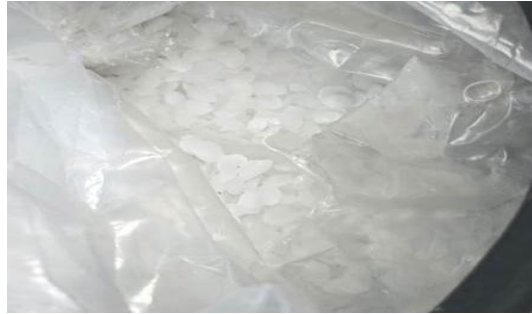
Fig. 4 NaOH in pellets form
