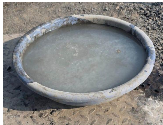
Fig.5 Na 2 SiO 3 in gel Form
