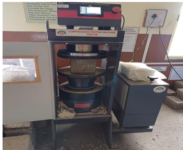
Fig.15 Testing of Compressive Strength using 2000KN compression testing Machine
