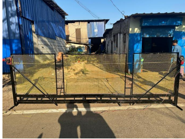
Fig. 9. Fabricated full-scale prototype, front view, in the raised (blocking) position.
