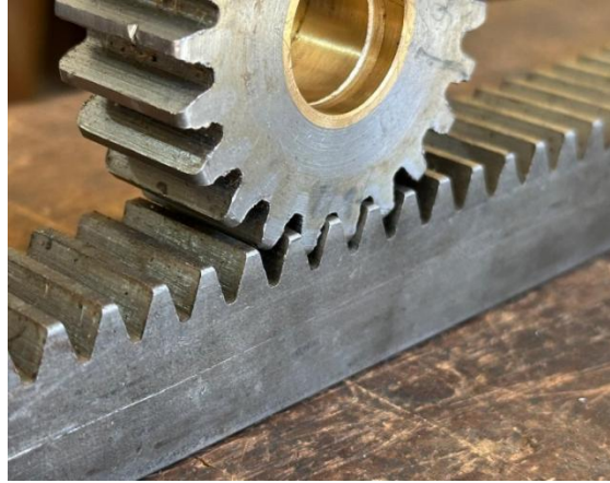
Fig. 5. Fabricated pinion meshed with the machined steel rack.
