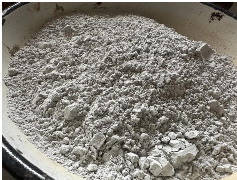
Fig. 1. Ground steel slag as received, showing the fine grey powder
