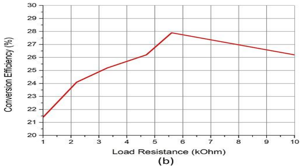
Figure. 3: Conversion efficiency of the half-wave rectifier.
