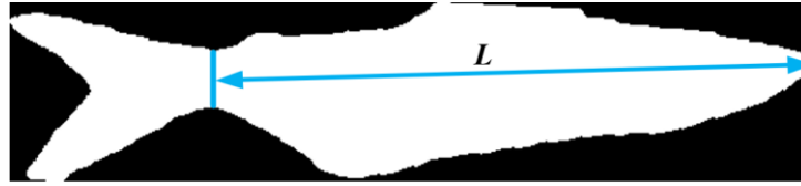
Fig. 7. Fish length measurement based on the extracted mask image.
