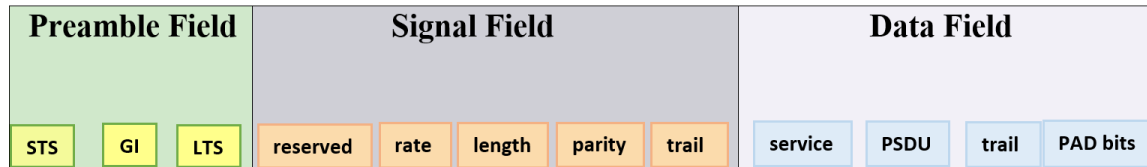
Figure 2. IEEE 802.11p PHY PPDU frame structure
