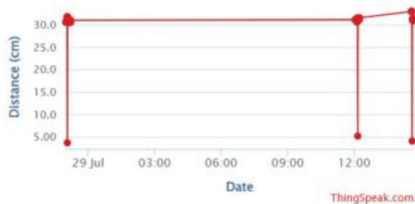
Fig. 3.1 – Variation of Waste-Surface Distance with Date and Time
