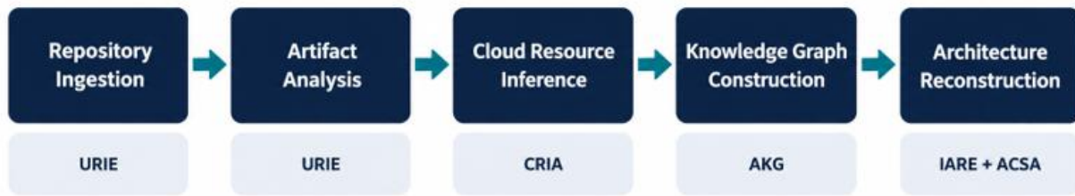
Figure 1. CloudBlueprintAI five-stage pipeline: Repository Ingestion → Artifact Analysis → Cloud Resource Inference → Knowledge Graph Construction → Architecture Reconstruction.
