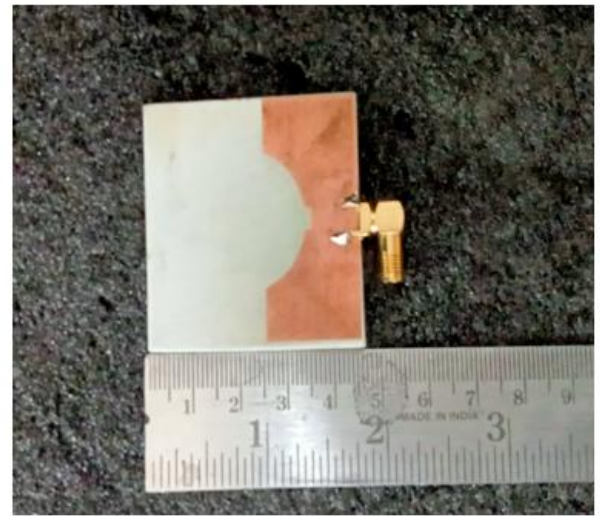
Fig. 19(b). Back view of the fabricated antenna.
